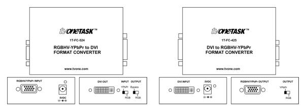
To begin, connect the AC adapter to the Format Converter's power input. Next connect the appropriate cable to the source device and then the Format Converter. Finally, connect the output cable to the Format Converter and to the destination device. Once the cables have been connected, you can apply power to the source and destination devices and then plug the Format Converter's AC adapter into the AC power source. The Format Converter will begin to function as soon as it has power.
