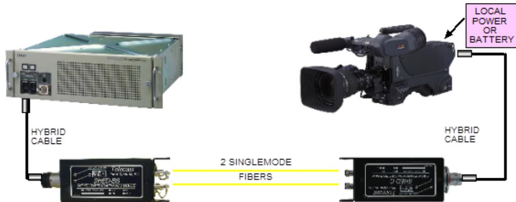
Fig. 2-1: Passive SHED-SHED System
