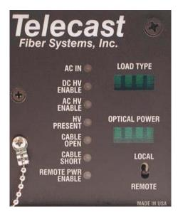
Fig. 3-1: HDX Front Panel Displays
