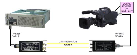
Fig. 2-1: Passive SHED-SHED System
