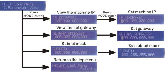
2. Display and adjust the operating parameters
