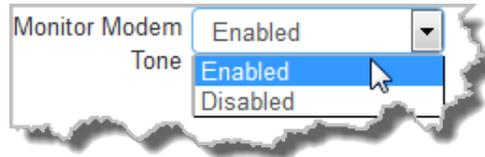
When enabled the module will allow audio monitoring of modem tones during connection in **POTS Codec** mode via the phone input. By default, the following phone input monitoring rules apply when multiple POTS G5 modules are installed in a codec and multiple POTS connections are dialed.
