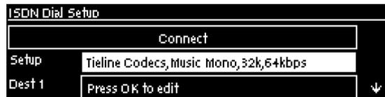
3. Select **Session Type [Sessionless]** > **Select Dial Route [None]** > **Number of B Channels [Choose the number of B-channels (between 1 and 4) required for your connection]** > **Algorithm [Choose G.722, E apt-X Mono or Stereo, MP2 Mono or Stereo or MP2 J-Stereo (Note: select 32kHz or 48kHz sample rate for MP2 depending on available B-channels)]**.
