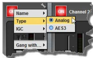
3. When you select AES3, the display changes to reflect 100% input levels; slider and input on/off controls are locked on.
