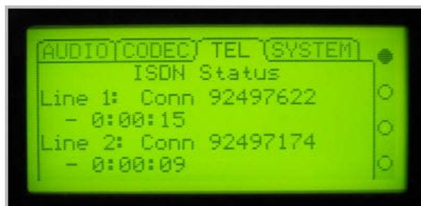
**Two ISDN B Channels Connected**
