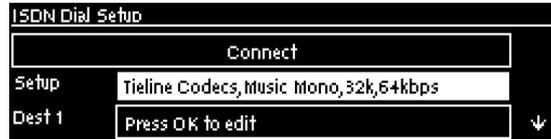
3. Select **Session Type [Sessionless]** > **Select Dial Route [None]** > **Number of B Channels [Choose 1B (mono) or 2B (stereo)]** > **Algorithm [Choose MP2 Mono or MP2 J-Stereo (Note: select 48kHz sample rate for MP2 algorithms)]**.
