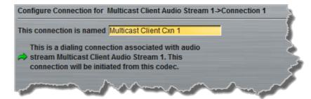
5. Follow the instructions on the right-hand side of the panel to configure the transport settings for the connection, then click **Next**. Note: select **UDP/IP +RTP** for RFC compliant streaming.
