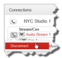
3. Click the connection **Connect/Disconnect** symbol to disconnect an individual audio stream connection.
