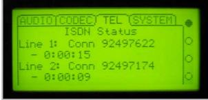
Two ISDN B Channels Connected
