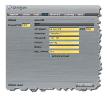
6. Navigate to **SETTINGS** → **SIP** > **Accounts** to verify that the account has been registered to the SIP server. The registration symbol appears when it is activated successfully.
