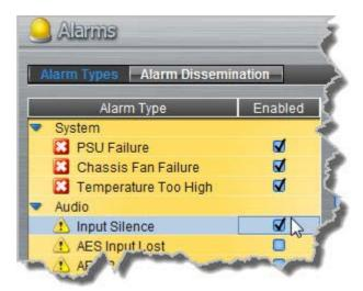
Configure the dBFS threshold and timeout duration in seconds within the Conditions pane and ensure the input check-boxes are selected. An alarm will be raised when these thresholds are breached.
