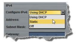
DHCP IP addresses are automatically assigned and can change each time you connect to your Internet Service Provider or to your own local area network (LAN). By default the codec is programmed for DHCP-assigned IP addresses.
