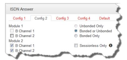
Configure the bonding setting that best suits the audio stream with which this Config is associated. Bonded or Unbonded is the best setting in most situations.
