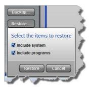
6. Click **Restore** to copy the configuration file settings onto the codec; confirmation of successful file restoration is provided.
