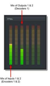
When connecting with a stereo program, the codec displays audio on **PPM1** and **2** for inputs 1 and 2 and **PPM 3** and **4** for the return audio.
