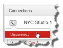
2. Click the audio stream **Connect/Disconnect** symbol and then click **Disconnect** to disconnect an individual audio stream and all associated connections.
