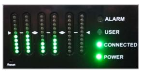
Stereo connection with PPMs 1-4 displaying input and return audio
