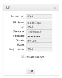
7. Navigate to **SETTINGS**  $\longrightarrow$  > **SIP** > **Accounts** to verify that the account has been registered to the SIP server. The registration symbol  $\checkmark$  appears when it is activated successfully.
