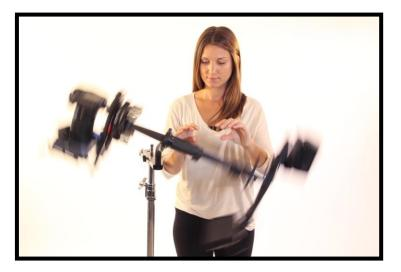
While on the balance pin, rotate the Sled to horizontal.
