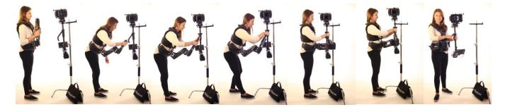
With the Docking stand raised so the Stage is roughly shoulder high, bow to the stand and place the Arm Post into the receiver of the Gimbal Handle.
