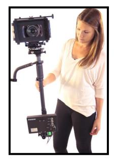
Fine tune this axis by turning the Side-to-Side Knob one way or the other to bring the camera completely level.
