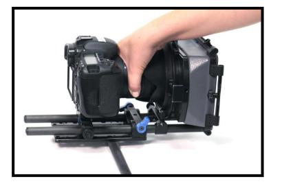
Rotate the camera  $90^{\circ}$  to the rod and find the Fore-Aft balance point using the same method.
