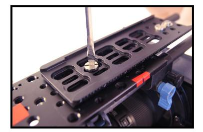
Fasten with the appropriate camera screw in the nearest opening. Do not over tighten, but ensure the camera will not rotate.
