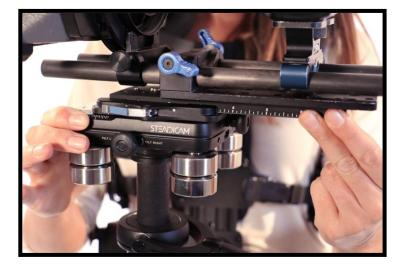
Once the AERO is in Dynamic Balance it's easy to maintain despite later changes to camera setup.
