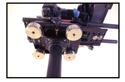
If your camera is especially light, you should consider adding weight through accessories like a larger battery or audio receiver.
