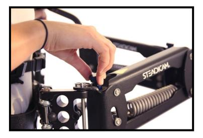
Repeat the adjustment on the Upper Arm section in the same way. Both Arm sections should move together when booming up and booming down. Test it to see.
