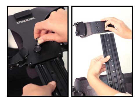
Flip the Plate over so the Socket is on the LEFT side of the Vest and reassemble.
