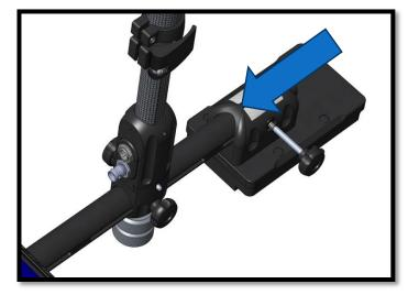
Second, remove the Battery Mount Locking Shaft, slide the Battery Mount onto the Rod and reinstall the Battery Mount Locking Shaft.
