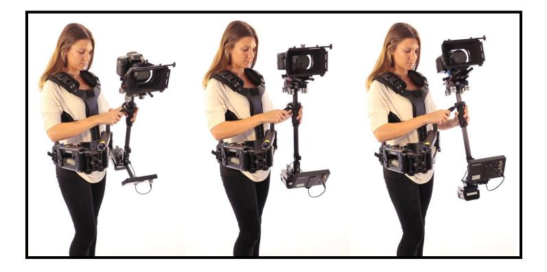
**In addition to helping balance the AERO Sled,** the Balance Weights and extendable Post allow adjustment of inertia and lens height to help you achieve each specific shot. Inertia is resistance to acceleration; the more inertia we have across each axis of our Steadicam, the more resistant the rig is to pan, tilt or roll. In combination with adjusting Drop Time, you can tune the AERO to be quick handling and active or slow handling and stable to suit each shot.
