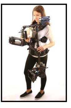
**A Steadicam Sled is in Dynamic Balance** when the Center Post remains vertical while the Sled is panned. Dynamic Balance is extremely important for precise operating, especially whip pans. For a detailed explanation of the physics of panning a Steadicam, look to the Steadicam Operator's Handbook. For every combination of camera, batteries, Post length and Balance Weights, there are multiple positions which will be in Static Balance but only **one** of these will be in Dynamic Balance.
