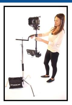
Set up the Docking Bracket on a stand and use a sand bag or a friend to keep it from toppling while the rig is on the balance pin.
