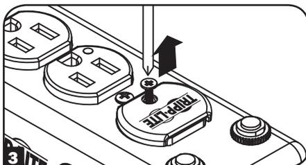
Save the cover and screw as it is designed for repeated use.
