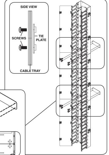
**Step 7** (Optional) Repeat Steps 1-6 to install another set of cable trays on the other side of the rack. (A single-depth installation on both sides of the rack requires 2 x SRCABLEVRT6 or SRCABLEVRT12.)
