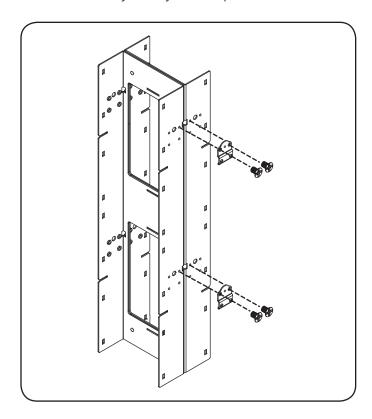
**Step 2** Using (2) M4 x 12 mm pan head screws, attach (2) mounting buttons to the mounting brackets.
