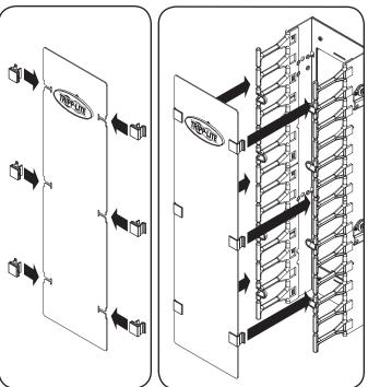
**Step 5** Align the mounting buttons with the toolless mounting slots on the side of the rack. Insert the mounting buttons through the slots and slide the cable tray downward until secure. Use (4) M4 x 12 mm pan head screws inside of the rack rail to fasten the cable tray in place.
