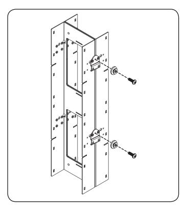
**Step 3** Attach (8) cable guides to the cable tray frames. The cable guides slide over the edges of the cable tray frames to form a tight attachment.
