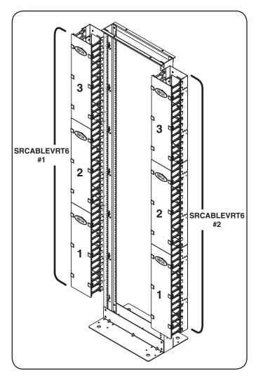
Note: SRCABLEVRT6 is shown. The cable tray frames and doors of the SRCABLEVRT12 are wider, but installation is identical.
