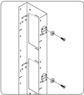
**Step 3** Attach (4) cable guides to the cable tray frame. The cable guides slide over the edges of the cable tray frame to form a tight attachment.
