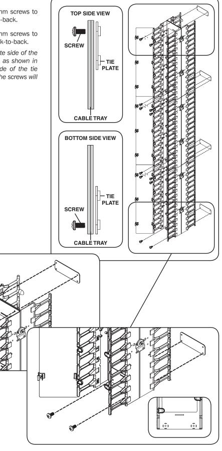
**Step 7** (Optional) Repeat Steps 1-6 to install additional cable trays on the other side of the rack. (A double-depth installation on both sides of the rack requires 4 x SRCABLEVRT6 or SRCABLEVRT12.)
