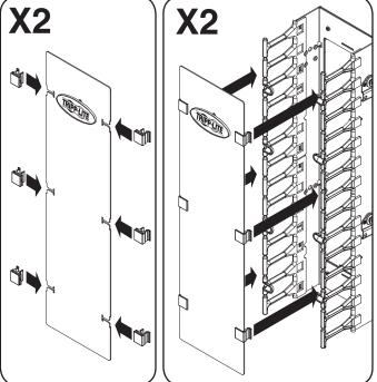
**Step 5** Align the mounting buttons with the toolless mounting slots on the side of the rack. Insert the mounting buttons through the slots and slide the cable trays downward until secure. Use (4) M4 x 12 mm pan head screws inside of the rack rail to fasten the cable trays in place.
