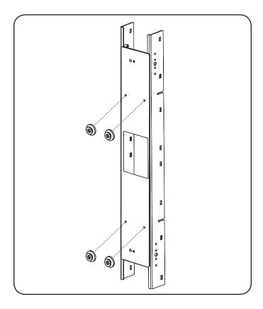
**Step 3** Attach the (4) cable guides to the cable tray frame. The cable guides slide over the edges of the cable tray frame to form a tight attachment.
