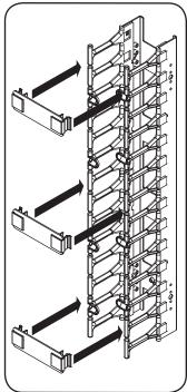
**Step 5** Align the mounting buttons with the toolless mounting slots on the enclosure's PDU manager, so that the SRCABLEVRT3 is facing the center of the rack. Insert the mounting buttons through the slots and slide the cable tray downward until secure.
