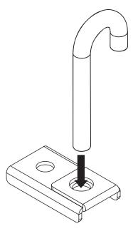
**Step 2.** Wrap the J-Hooks and clamps around the frame of the ladder. The other side of the clamp (without the J-Hook installed) will wrap underneath the perpendicular frame on the 4-post rack. Tighten this system by securing the J-Hook to the Adjustable J-Hook Clamp using the included M8 Washers and M8 Hex Nuts. Repeat this procedure for the other side of the ladder frame, if making attachments between two 4-post racks.
