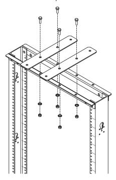
**Step 2.** To attach the ladder, extend the SRCABLELADDER between your two intended racks (or wall) and attach the ladder to the Perpendicular Junction Plate by hooking two J-Hooks around the ladder frame and into the outside holes on the Junction Plate. Secure the two hooks using two of the included M8 Washers and M8 Hex Nuts. *Note: Diagram shows installation of two separate SRLADDERATTACH and SRCABLELADDER units.*
