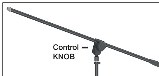
Boom has “4 Degrees of Freedom”. The boom adjusts front-to-back, up-and-down, side-to-side and rotationally. Simply untighten the control knob, make all four adjustments and tighten snugly. To telescope, use smaller knob along boom shaft to adjust the length.
