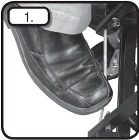
**STEP 1:** Apply pressure to release cable with foot or hand.
