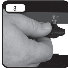
**STEP 3:** Tighten spring-loaded wing nuts.
