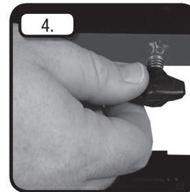
**STEP 4:** Tighten spring-loaded wing nuts.
