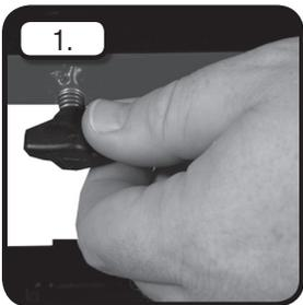
**STEP 1:** Loosen spring-loaded wing nuts.
