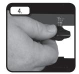
**STEP 4:** Tighten springloaded wing nuts.
