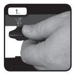
**STEP 1:** Loosen springloaded wing nuts.
