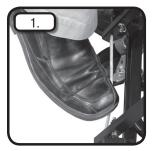
**STEP 1:** Apply pressure to release cable with foot or hand.
