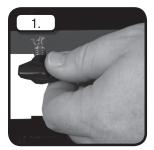
**STEP 1:** Loosen springloaded wing nuts.
