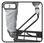
**STEP 2:** While applying pressure to release cable, raise foldable side to upright position.
