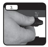
**STEP 3:** Tighten springloaded wing nuts.
