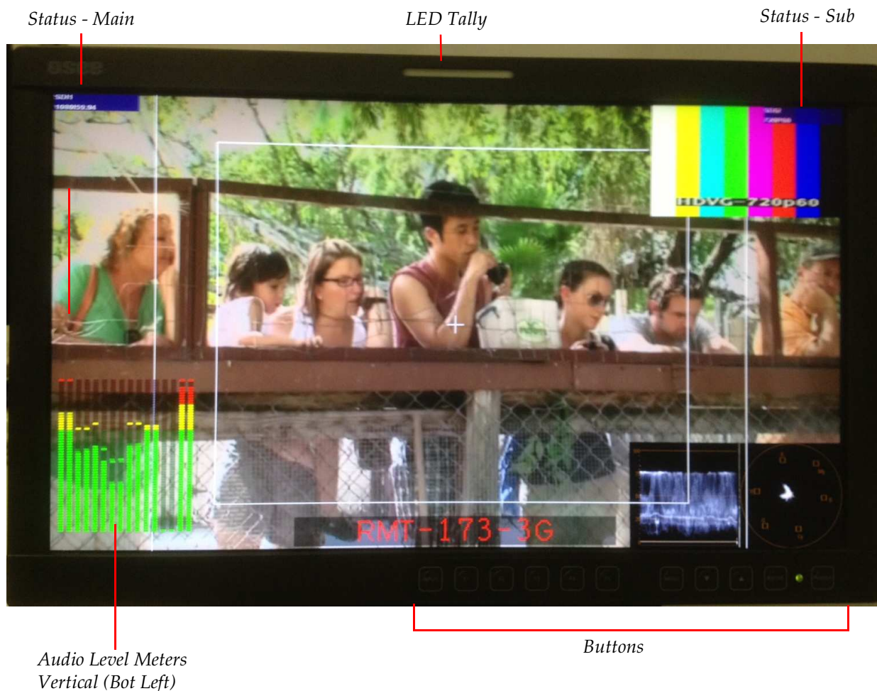
Figure 1–3 RMT-173 Front Panel (PIP Layout)
