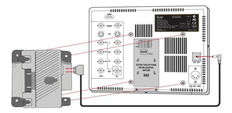
Attach the Pro Battery Plate to the VX9 monitor with four M4X.07 20mm Bolts.
