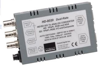
The 8020 is a compact HD/SD dual-rate digital to analog converter. The 8020 supports SMPTE-292 1080i, 720p and SMPTE 259M-C 525/625 SD signals. HD signals are converted to HD YPbPr or GBR wide band HD analog signals with H/V or embedded tri-level sync. SD signals are converted to SD analog component, composite and Y/C with embedded sync. User programmable overlay reticules are available on both HD and SD outputs. All conversions are 12-bit encoded from 10-bit input video resolution.
