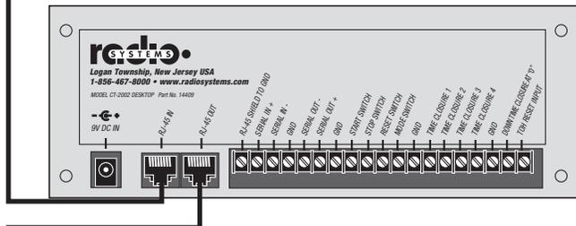
Use a crossover RJ-45 patch cable to slave Time-of-Day and/or timer displays to downstream units.
