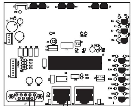
Serial daisy chain connectivity may also be via CAT-5 cable and RJ-45 connectors. Use a standard 568B ethernet patch cable (all wires connecting straight thru pin to pin) or for custom made cables observe pinouts to right.
