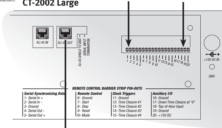
Use a straight thru RJ-45 patch cable (from either RJ-45 connector) if this clock is being fed with remote master time sync and if downstream displays are not required to display remote timer information.
