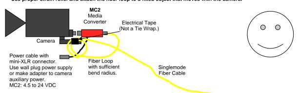
3) DO NOT USE. Avoid strain and motion on fiber connector.
