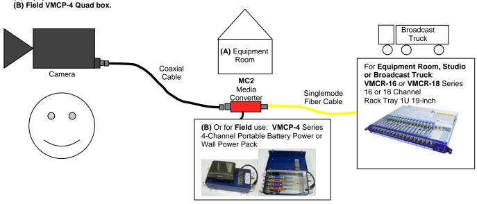
2) If must mount to a camera, USE FIBER LOOP to avoid strain and motion on fiber connector.
