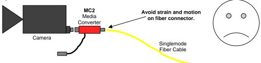
NOTE: Always use good fiber cable management, follow fiber bend radius recommendations and use appropriate strain relief techniques.
