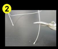
Take some wire snips and cut off about 2 1/2" inches of wire on the right side (boom side). Make sure you take off the rubber tip to use in step 3.
