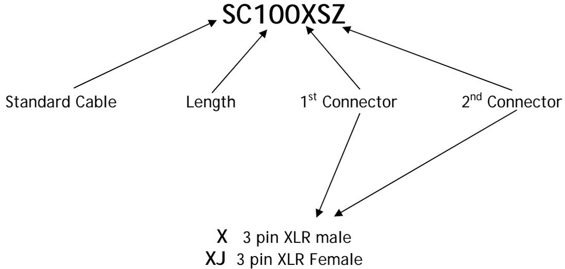
**S** ¼" Phone Plug (male) TS Tip / Sleeve 2 Conductor, Mono, Unbalanced
