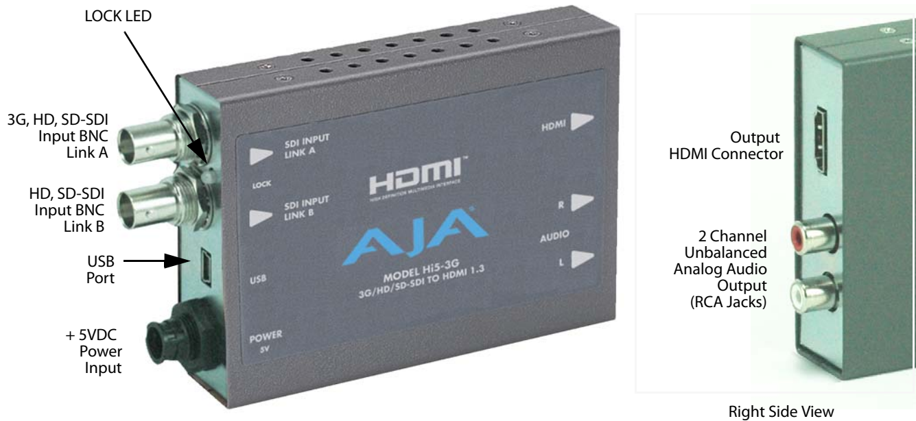
Figure 2. Hi5-3G Connections
