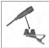
Fig. 2: Fixing the microphone on the clip.
