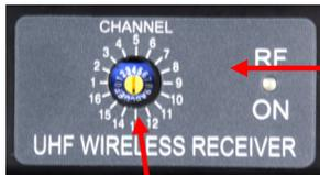
**16. Wireless 16 Channel Selector (left side of case)**—rotate knob to select wireless channel on the built-in receiver. RF LED will light up when receiving signal from transmitter.
