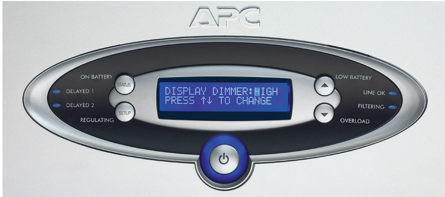
Figure 21. DISPLAY DIMMER (HIGH) Setting Screen
