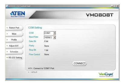
The controller's serial port should be configured as follows:
