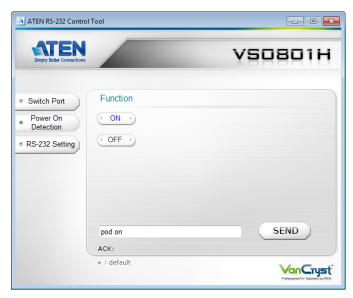
The Power on Detection page is used to enable or disable the Power on Detection feature. Power on Detection is used to automatically switch to the next port with a powered on device, when the current port device is powered off. The Power on Detection feature is turned off by default.
