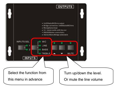
For example, to turn up the line volume, you should select the "LINE" first, and then press the button ".
