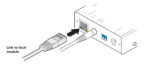
Figure 3-10. Attaching the CATx link cable
