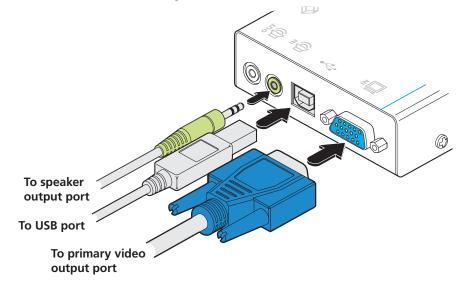
Figure 3-3. Attaching the video, USB and (optional) audio cables
