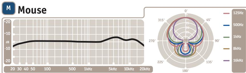
This frequency chart of the Mouse capsule is only a start. It gives the recordist a basis of the sound provided. How the microphone reacts in a particular application will differ greatly because of many variables. Room acoustics, distance from sound source (proximity), tuning of the instrument and microphone cabling are only a few of the interacting issues. For an artist or engineer, how the microphones are used creates the basis of the sound.
