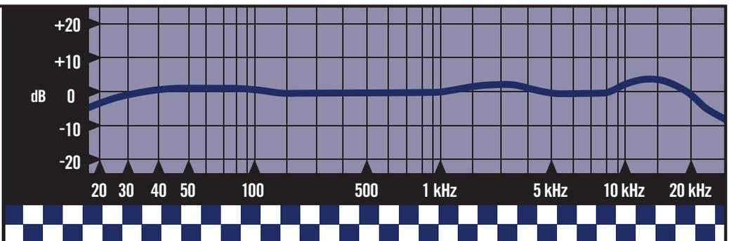
This frequency chart of the Stage Two B8 capsule is only a start. It gives the recordist a basis of the sound provided. How the microphone reacts in a particular application will differ greatly because of many variables. Room acoustics, distance from sound source (proximity), tuning of the instrument and microphone cabling are only a few of the interacting issues. For an artist or engineer, how the microphones are used creates the basis of the sound.
