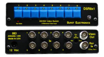
On the rear panel of the DSR8x1, the Ref Input port can be configured as a secondary video output. To
