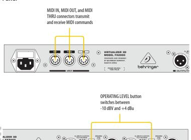
INPUT and OUTPUT connections are available as balanced 1/4" TRS and XLR jacks
