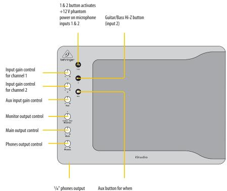
Aux button for when a turntable is connected to the Line/Phono Aux RCA inputs
