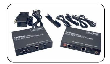
The CableTronix CT-HDBASET-330 is a five play signal extender which utilizes a single Cat5E/6 cable. The unit is capable of transporting HDMI signals, Ethernet, IR remote control signals, RS-232 Control, and PoE power all over one CAT5E/6 cable. This easy to install system allows for transmission distances over twisted pair up to 330 feet.
