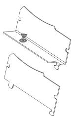
Your DA-506BID is supplied with extra mounting ears. These allow the DA-506BID to be mounted in any OpenHouse™ structured wire grid system.
