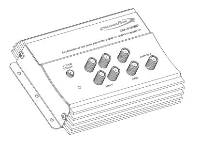
The DA-506BID video amplifier hub distributes CATV or antenna signals to 6 TVs. The DA-506BID has four short run outputs (up to 75 feet) and two long run outputs (up to 150 feet) for maximum flexibility. The DA-506BID has a broadband 54-806MHz amplifier and a 5-42MHz reverse channel which is compatible with pay-per-view, interactive cable and cable modems.
