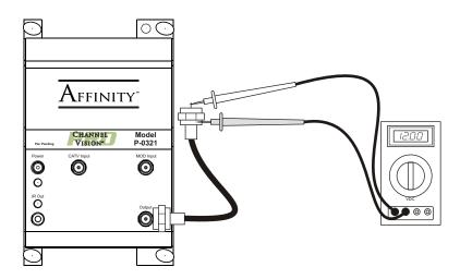
If you are using an RF splitter between the modulator and the P-0321 or between the P-0321 and the IR coax adaptor (IR-4101), check to make sure you have approximately 8-12 Volts DC on the coax going into the IR-4101. If there is no voltage at that point, check the following items:
