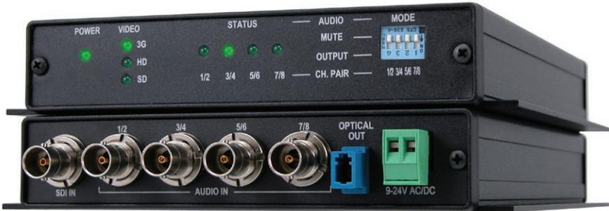
The Fiberlink® 3360 Series allows you to transmit 3G, HD or SD-SDI as per SMPTE 424M-2006, 292 and 259 with the ability to embed up to 8 channels (4 pairs) of AES/EBU digital audio. Convenient switches on the 3360 Series transmitter allow the operator to embed each of the four pairs of audio independently, to strip previously serialized audio, or to pass it through without modification. At the receive end of the fiber optic link, the operator can decide which audio pairs they need de-embedded.
