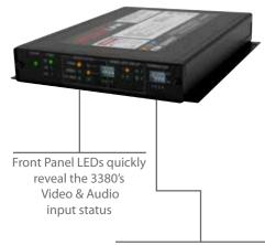
Dip Switches allow for quick configuration of your audio embedding preferences and audio termination
