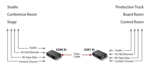
Bi-Directional Audio, Data, Ethernet, & Contact Closure on One Fiber
