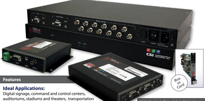
Supports VGA, SVGA, XGA and WXGA (640 x 480 up to 1366 x 768)
