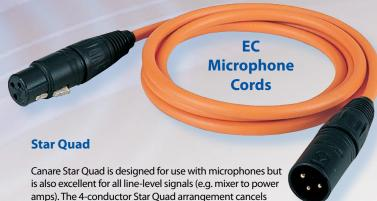
is also excellent for all line-level signals (e.g. mixer to power amps). The 4-conductor Star Quad arrangement cancels electromagnetically induced noise from SCR dimmer packs, fluorescent lighting ballasts and AC power transformers. Handling noise is prevented by use of cotton filler material. Excellent frequency response is maintained due to special irradiated polyethylene insulation which provides a low capacitance dielectric.
