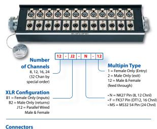
High quality ITT CANNON, JAE or DDK Multipin bayonet lock and XLR3 connectors are meticulously hand assembled and soldered with a minimum of unshielded wire leads.
