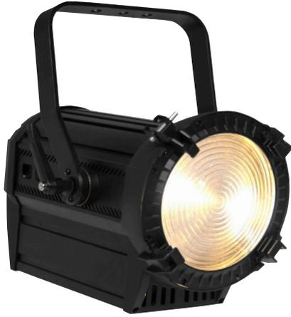
Powered by 16 10-watt LEDs, Ovation™ F-165WW delivers a smooth, even wash with a warm color temperature and a beautiful soft field. It also features an easily adjustable, motorized zoom with a range from 25° to 76° and can accommodate barn doors for glare reduction and beam shaping. Selectable dimming curves make it compatible with older, traditional theatre Fresnels.
