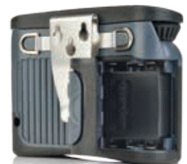
18+ hours of battery operation (door shown open)
