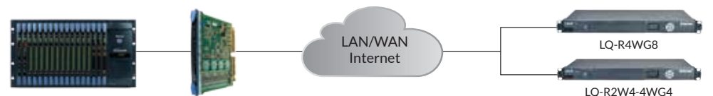
Linking matrix to GPIO, 2-wire or 4-wire intercom system
