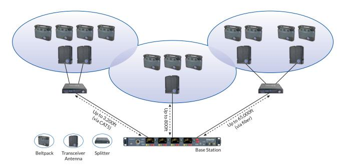
Expansive wireless coverage can be achieved by strategically placing up to 10 remote antennas across a wide coverage area. Each Transceiver Antenna can be positioned away from the base station or matrix up to 3,280 feet using a CAT5 connection or as far as 65,000 feet using a fiber connection. Each powered Antenna can create a coverage zone of up to 300 ft (indoor) or up to 800 feet (outdoor).
