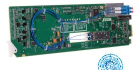
The 9214-2EO is dual SDI to fiber optic transmitter card. The card converts two SDI signals to two fiber optic links, allowing for longer transport distances. Reclocked SDI outputs provide copies of each SDI input signal. The card supports serial digital data rates from 270 Mbps up to 2.98 Gbps (1080p). LED indicators at the front of the card identify the presence of incoming video and the identified signal data rates for each channel independently.
