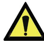
The exclamation point triangle is used to alert the user to important operating or maintenance instructions.
