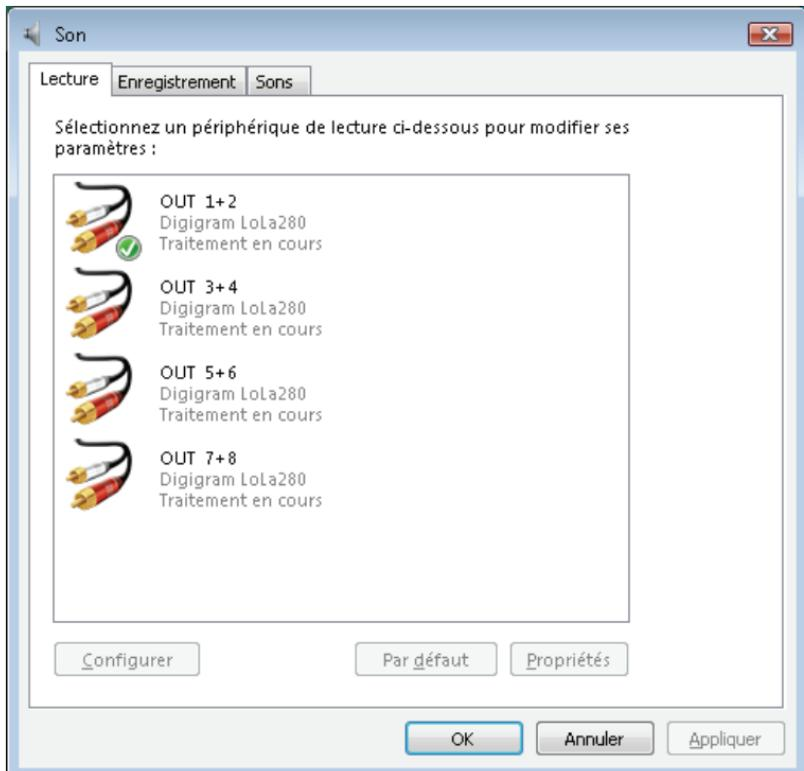
The DirectSound devices in playback mode correspond to the “**Playback**” inputs of the mixer. The manager allows mixing the corresponding streams on the two analog outputs.
