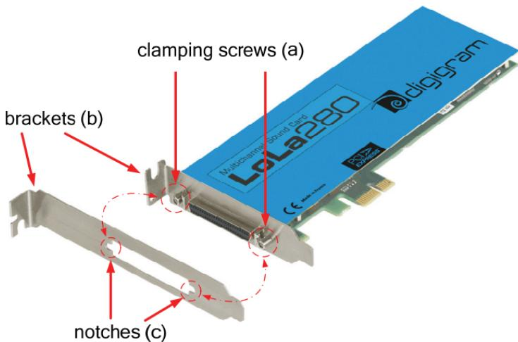
Unscrew the clamping screws (a), then remove the bracket (b) from the card and replace it by the one to be used, positioning it in the same sense on the card. Re-fasten the clamping screws using the notches (c) in the brackets.
