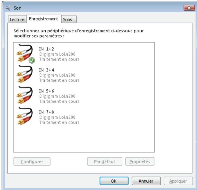
The DirectSound devices in recording mode correspond to the “**Record**” outputs of the mixer. The manager allows to send any combination of the eight analog input signals onto each one of these devices.
