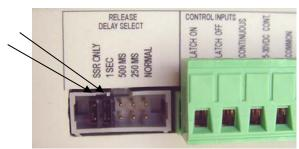
Example: Delay select jumpers shown for 1 sec. delay and Solid State Relay drive voltages only.
